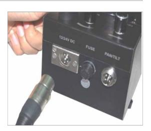
**CAUTION:** DO NOT USE A UNREGULATED POWER SUPPLY! IF USING A REGULATED POWER SUPPLY IT MUST PRODUCE LESS THAN 12 VOLTS. MORE THAN 24 VOLTS MAY CAUSE PERMANENT DAMAGE.
