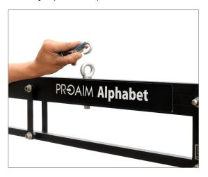
Similarly attach the second blue cable and align both the blue cables to the side of support rod.
