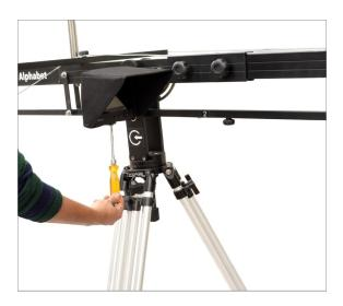
• The camera plate can be tilted upwards & downwards with the help of provided handle.
