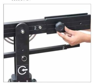
• Then tighten both the sections together using the provided knobs.
