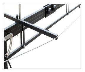
Now attach one end of 14.3ft red cable to red hook on back side of jib (section 3) and align the red cable to the cable guide from top.
